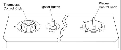
Figure 17 - Thermostat Control Knob In The OFF Position
